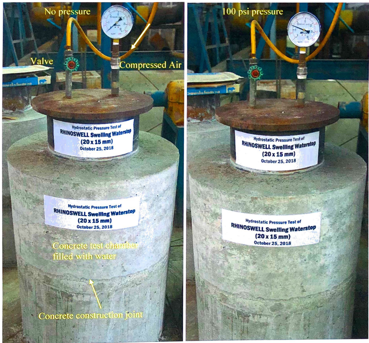
Photograph 3 – Completed concrete test chamber prior to the pressurization and at 100 psi (70.3 m water) pressure. No leakages at the joints were noted.
