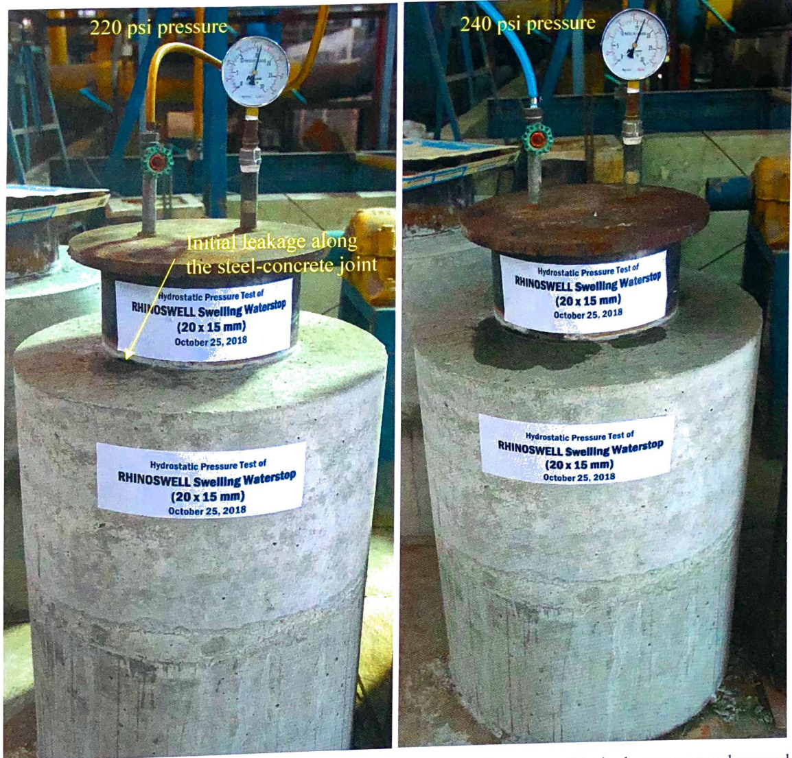
Photograph 4 – Concrete test chamber at 220 psi and 240 psi pressure. No leakages were observed at the concrete construction joints after one hour of tests. At the steel-concrete joint, initial leakage was noted at 220 psi pressure.
