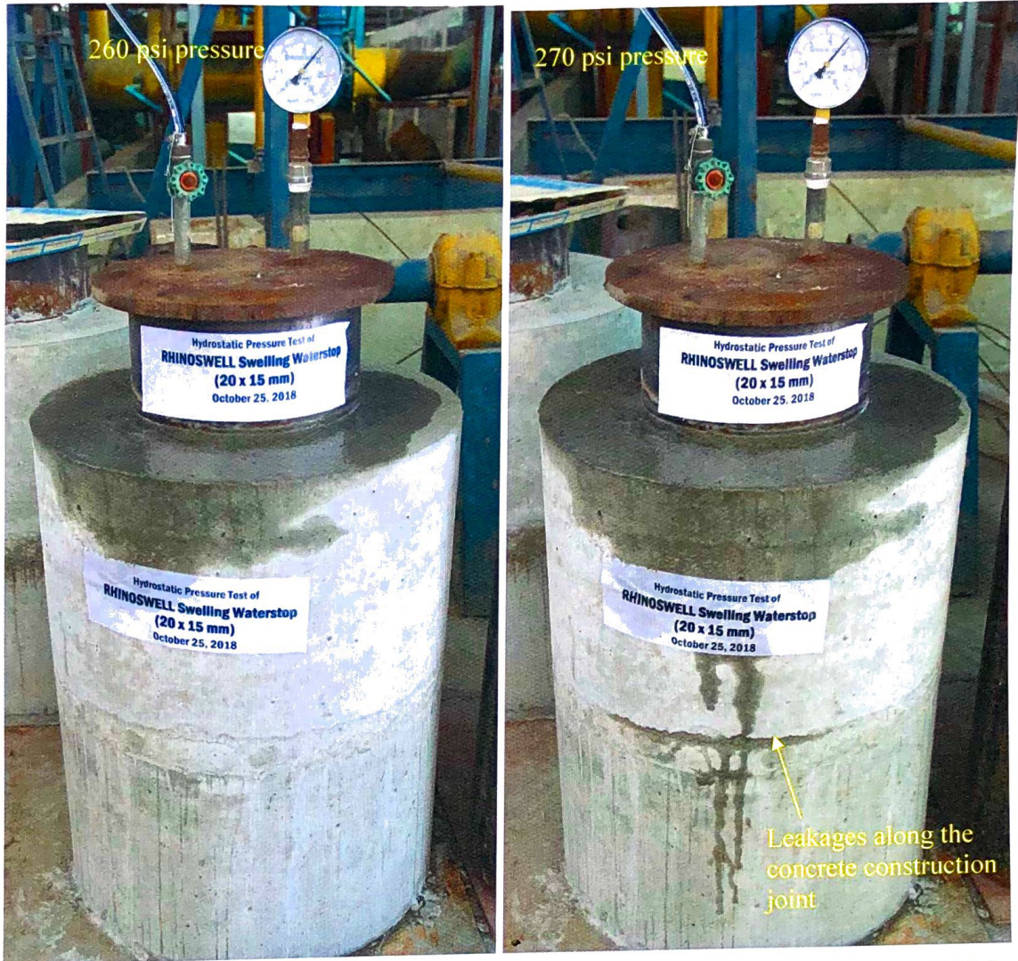
Photograph 5 – Concrete test chamber at 260 psi and 270 psi pressure. At 260 psi pressure (182.8 m water), no leakages were observed at the concrete construction joint. At the steel-concrete joint, leakages were noted. At 270 psi pressure (189.8 m water), initial water leakage was noted at the concrete construction joint. Therefore, the maximum effective pressure of RHINOSWELL Swelling Waterstop (20x15 mm) with RHINOLATEX adhesives to prevent water leakages along concrete construction joints is at 260 psi (182.8 m water) pressure.
