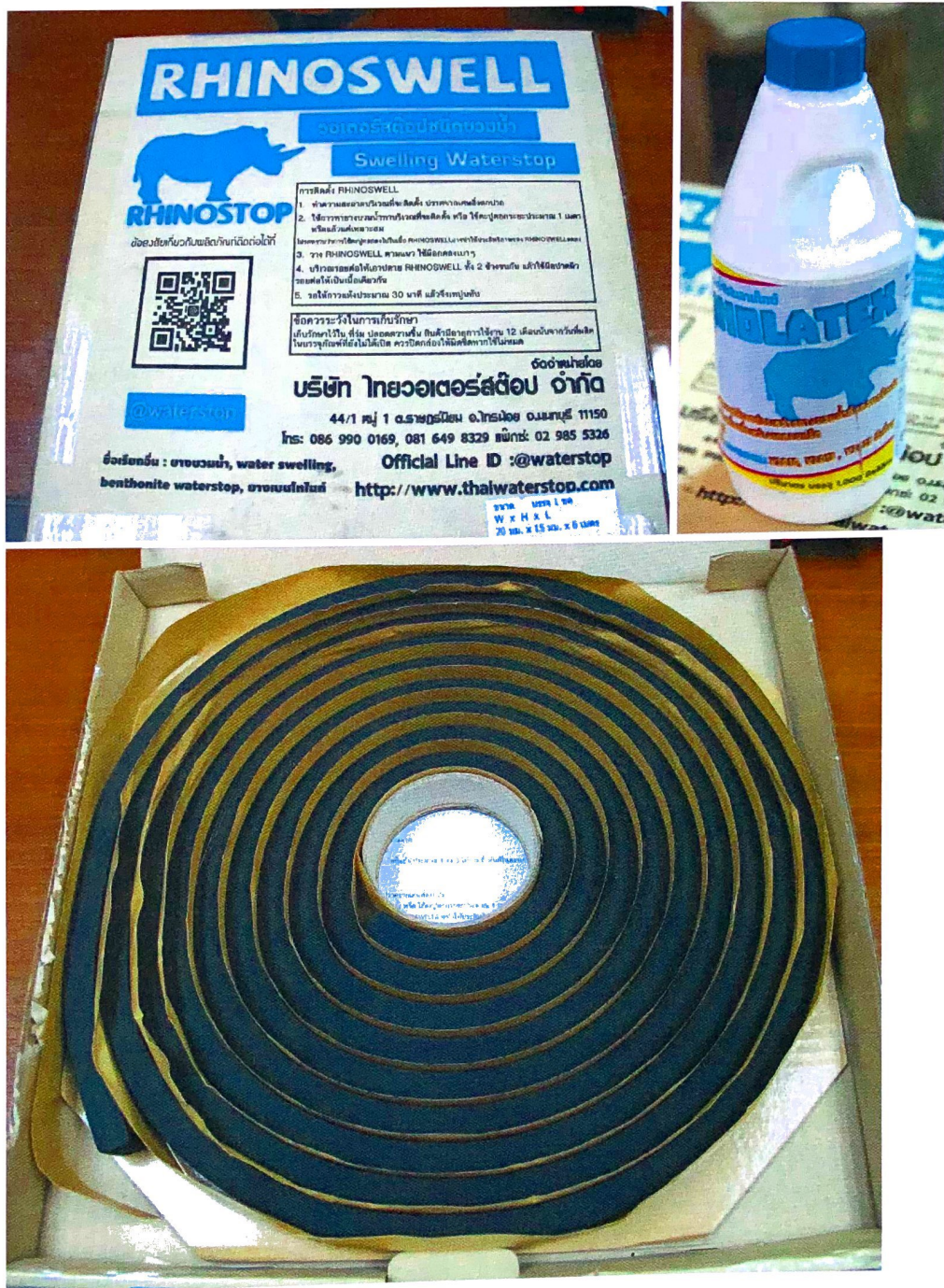
Photograph 1 – RHINOSWELL Swelling Waterstop (20x15 mm) and RHINOLATEX adhesives used in the laboratory tests.
