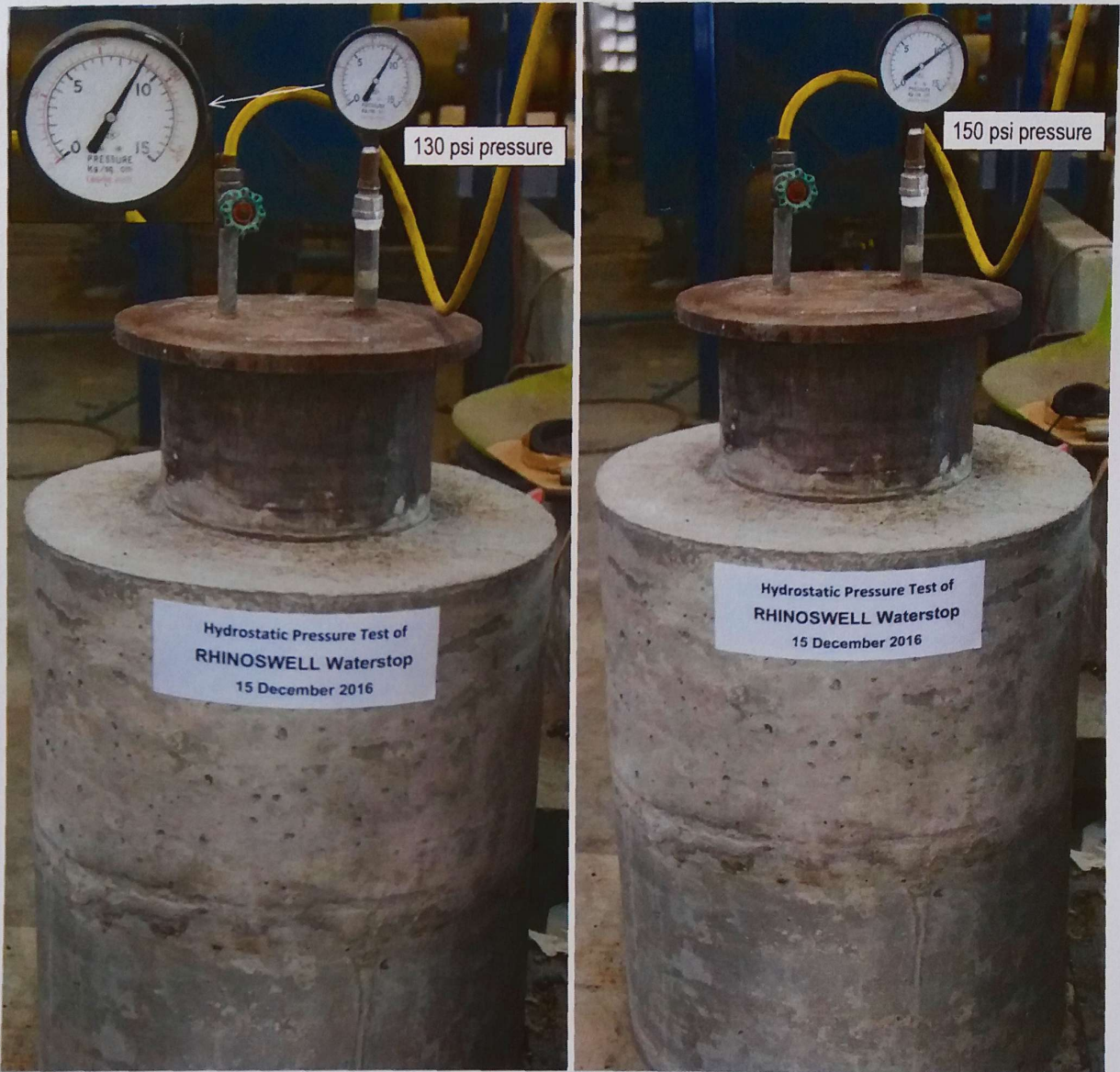
Photograph 4 – Concrete test chamber at 130 psi and 150 psi pressures. No leakages along the construction joints were noted after 1.0 hour of test for each pressure level.
