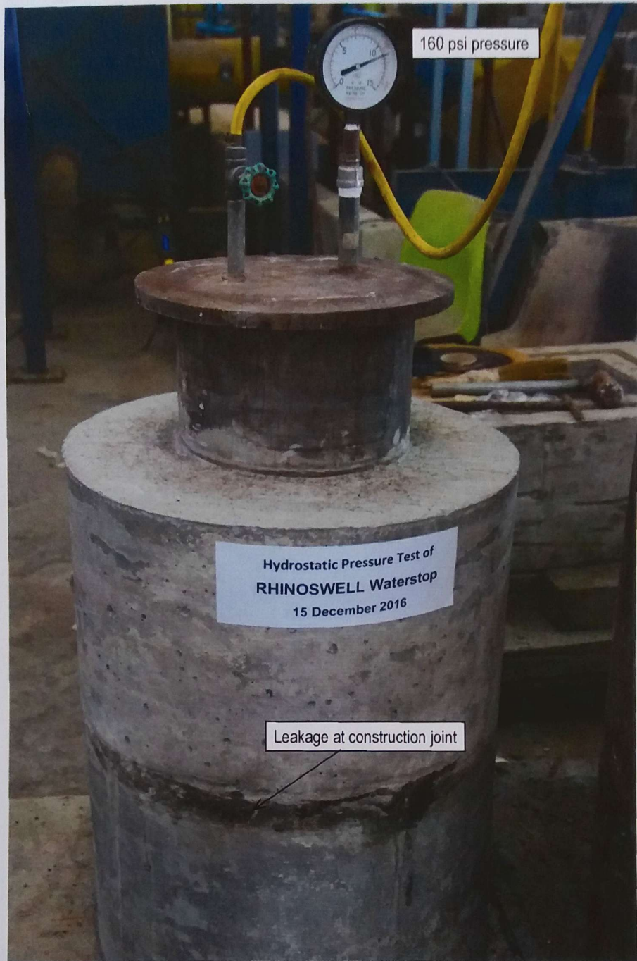
Photograph 5 – Concrete test chamber showing initial leakage at the construction joint after one hour at 160 psi (112.68 m of water) pressure.
