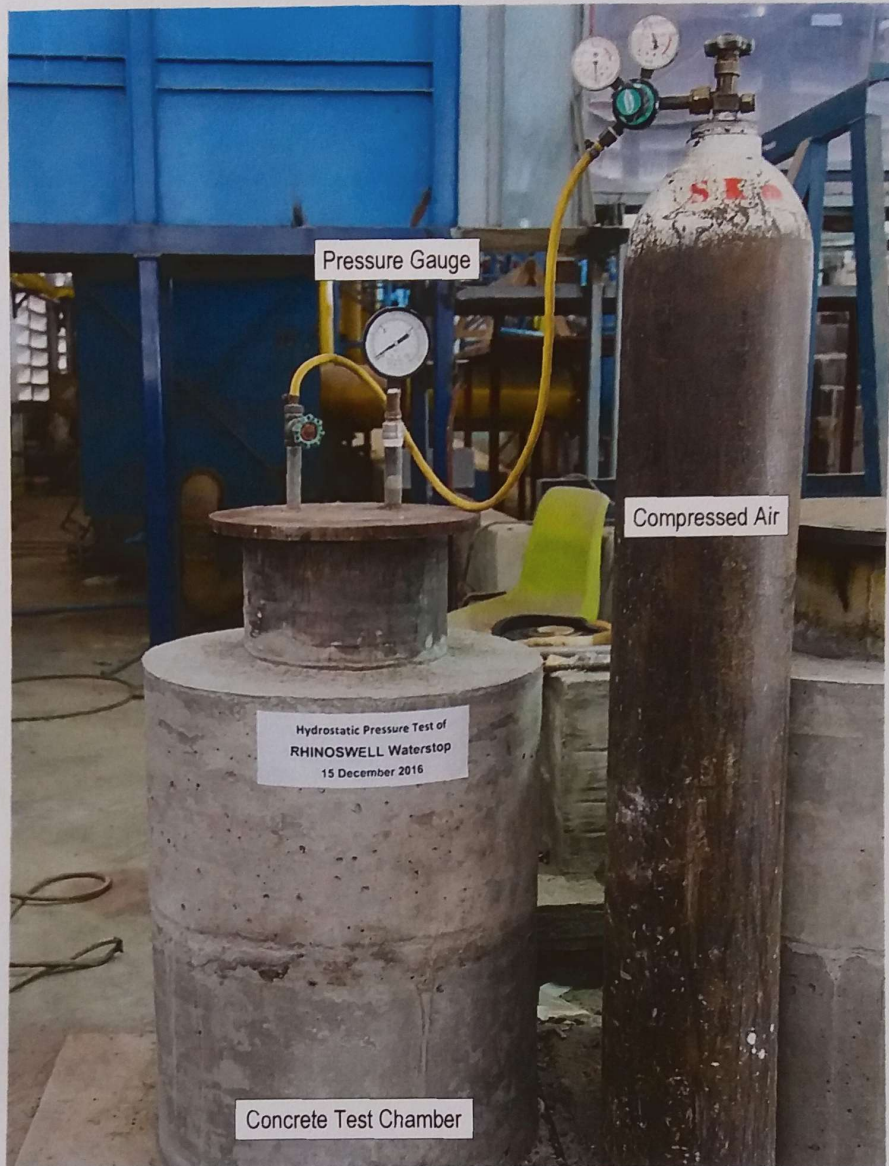
Photograph 3 – Completed set-up for the hydrostatic pressure tests
